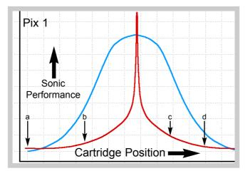
2/ The adjustments are very easy to misinterpret. Tweakers may expect easily heard sonic differences from every cartridge position change they make, assuming a "movement to result" curve as shown by the blue line in Pix 1 with steadily sloping sides and a wide flatish optimum. But the reality is that the actual curve is far more like the peaked red line, and this make the job a tad more tricky...
